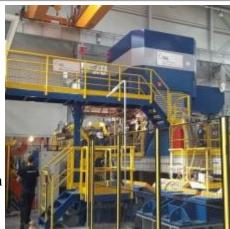
Equipped with the induction heating system for tight edges control, a new VOC emission control to guarantee low emissions, and a rolling oil recovery and distillation system, the mill is run by the Danieli FATA Hunter hSystem® to automatically control AGC and AFC and can roll a wide variety of products from foil stock to can body with best-in-the market tolerances and quality.
